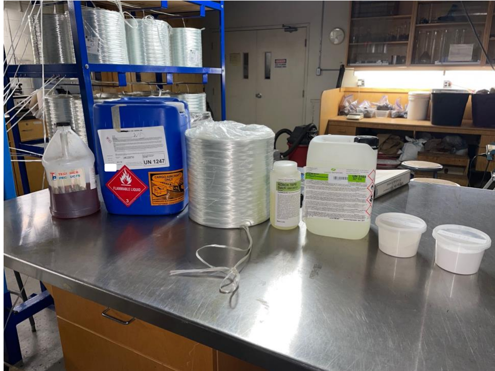
Figure 3.1: Materials used for pultrusion manufacturing. From left to right: lubricant, resin, glass fibre roving, initiators, and fillers.
