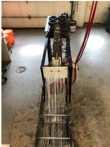
Figure 3.3: Top view of pultrusion set-up
