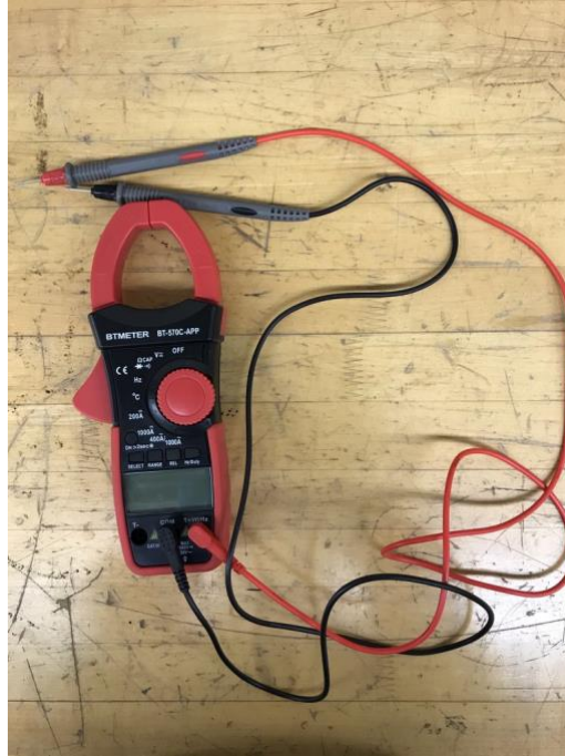
Figure 4.9: Clamp-meter for measuring current and voltage from pultrusion machine
