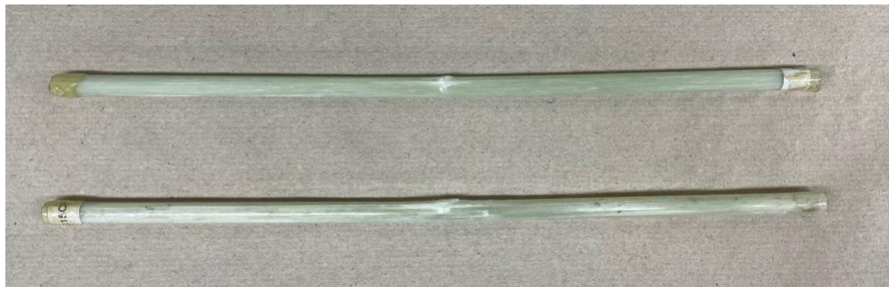
Figure 3.5: Lab-manufactured and -tested TP (top) and TS (bottom) GFRP specimens
