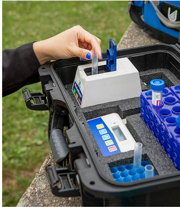
Figure 3: 2nd Generation ATP ® Testing Equipment (LuminUltra Technologies Ltd., 2024)
