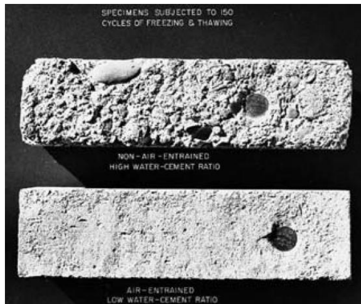
Figure 2.11 Non-Air-Entrained Concrete and Air-Entrained Concrete After 150 Freeze-Thaw Cycles (Kosmatka et al. 2002)
