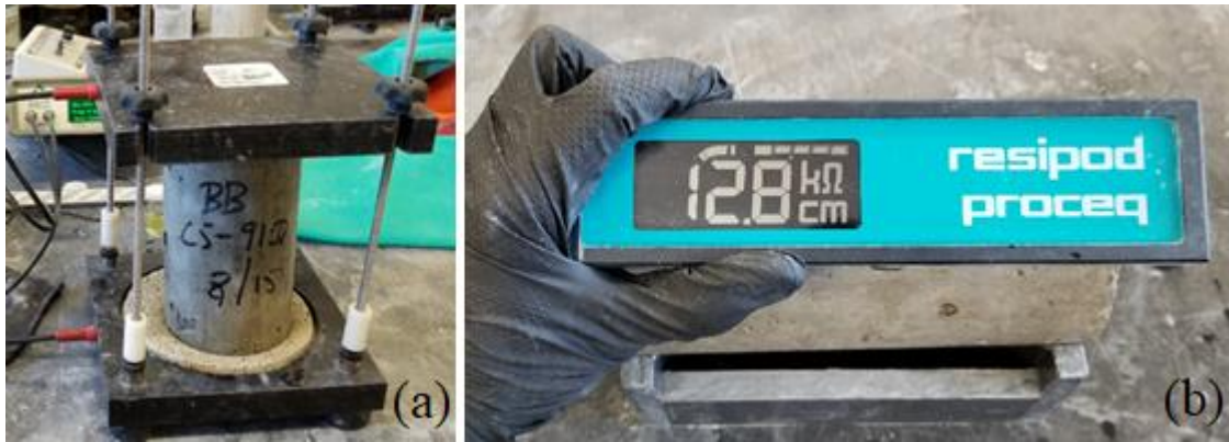
Figure 3.5 Measurement of (a) Bulk and (b) Surface Resistivity of a Concrete Specimen
