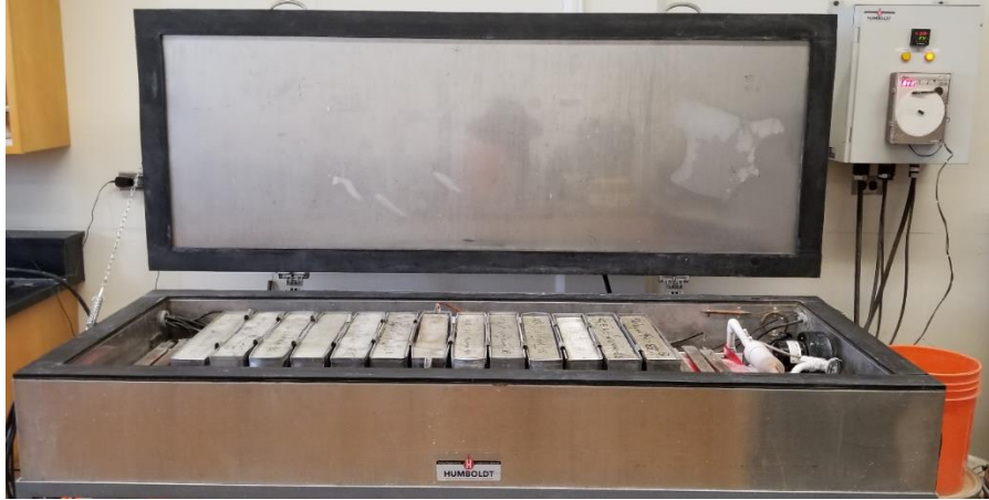
Figure 3.8 Specimen Arrangement in Freeze-Thaw Apparatus
