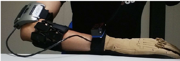
Fig. 4: Double MYO setup in Ninapro DB5 (image adopted from [36], under the Creative Commons Attribution License )
