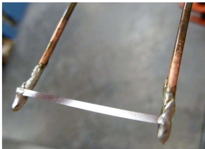
Figure 13 Picture of the Nichrome ribbon welded at the ends of two copper wires
