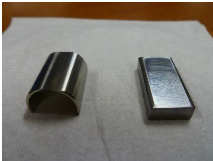
Figure 26 Polished metal samples used for contact angle measurements (Alloy-800 on the left, carbon steel A106-B on the right)
