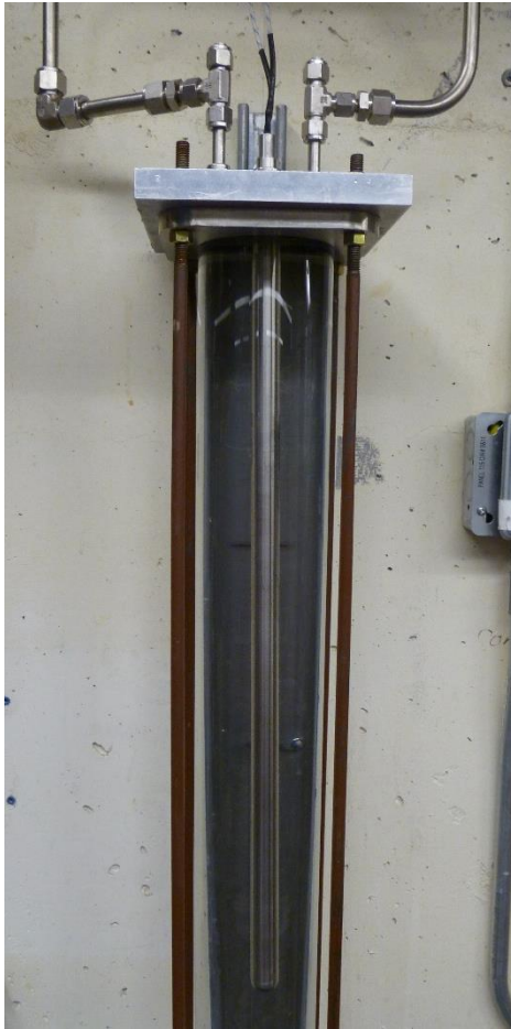
Figure 14 Picture of the recirculating loop test section
