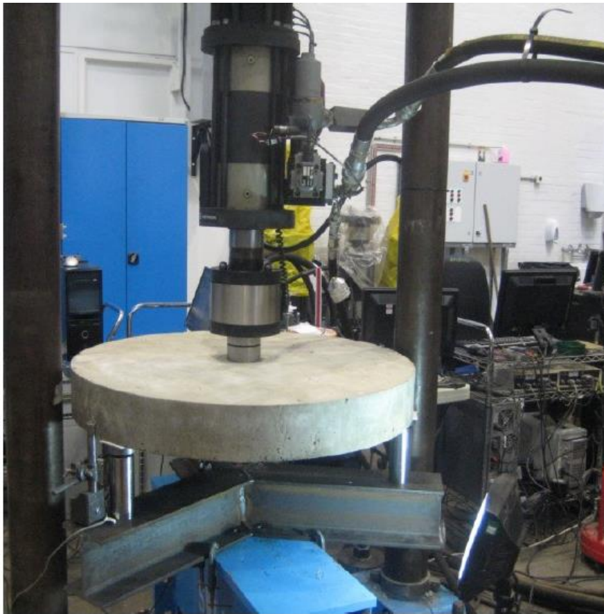
Figure 2.13: Photo of test set-up for panel test (Oikonomou-Mpegetis, 2013).
