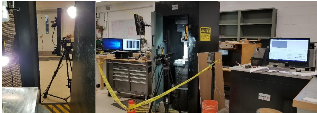
Figure 4.1: DIC test set-up.
