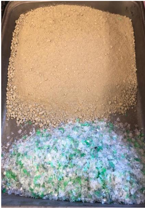
Figure 14. Shredded Plastic and Crushed Rock
