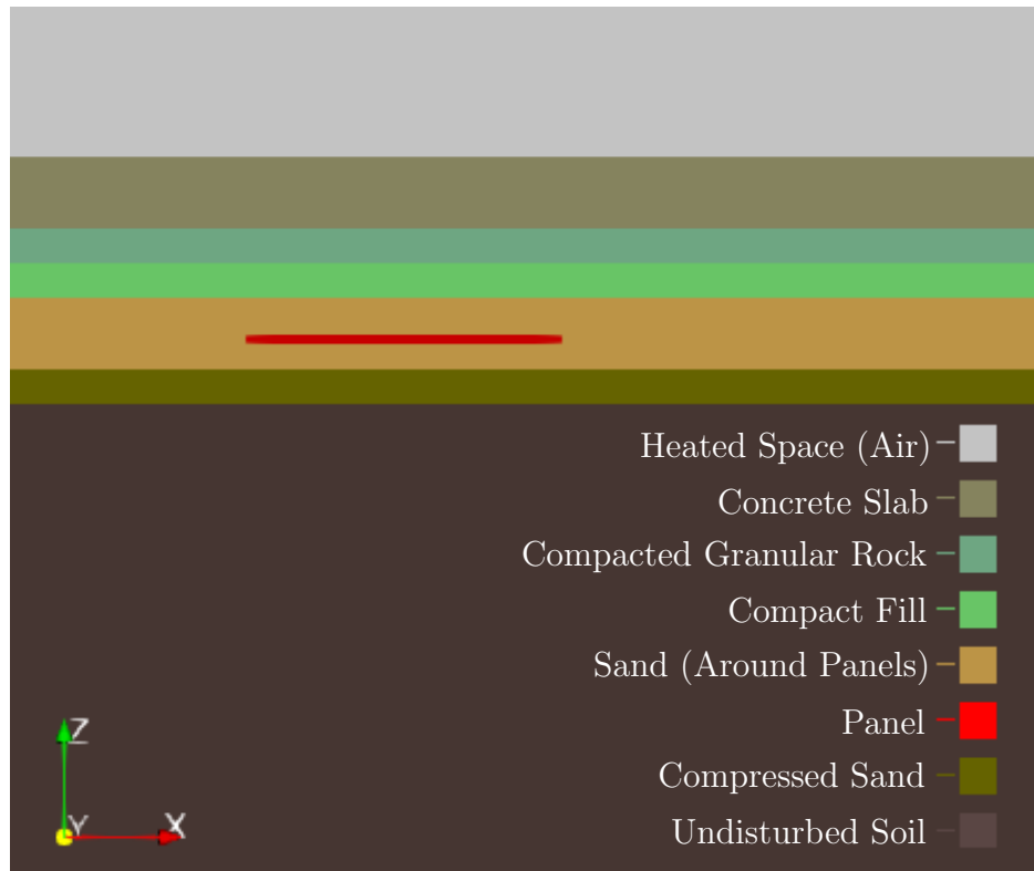
Figure 1.1: Cross-sectional View of ThermaRay's ESS [4]
