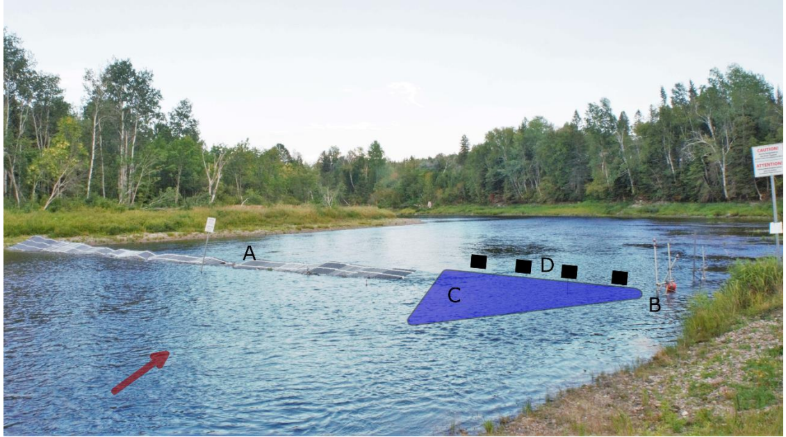
Figure 26. Study site at the Little Southwest Miramichi River. The Resistance Board Fish Weir (A) guides fish to one side of the river, where an ARIS sonar (B) is recording with 11.1 m end range (C) and four underwater cameras (D) are aimed to the middle of the river. The flow direction indicated with an arrow.
