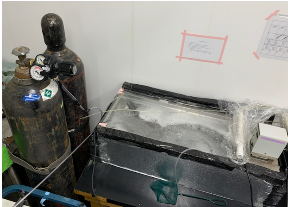
Figure 1: Water bath setup for acute hypoxia trials. Oxygen depletion was achieved by bubbling compressed nitrogen gas through two micro bubble diffusers. Temperature and dissolved oxygen levels were continuously monitored via a handheld probe.
