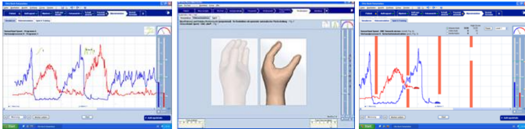
Figure 3-2: Ottobock PAULA training suite (raw muscle activity, prosthetic hand simulator, and car game, left to right)
