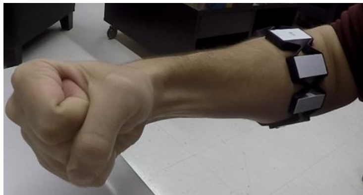
Figure 2-4: Co-contraction impulse (quick, simultaneous contraction of both the inner- and outer-forearm muscles)
