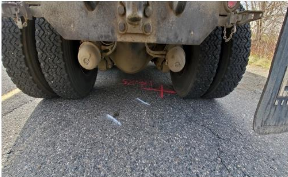
Picture 4. NBDTI Vehicle - Loaded Plow Truck at Static Location 10 – Rear Tandem Axle over Crown.
