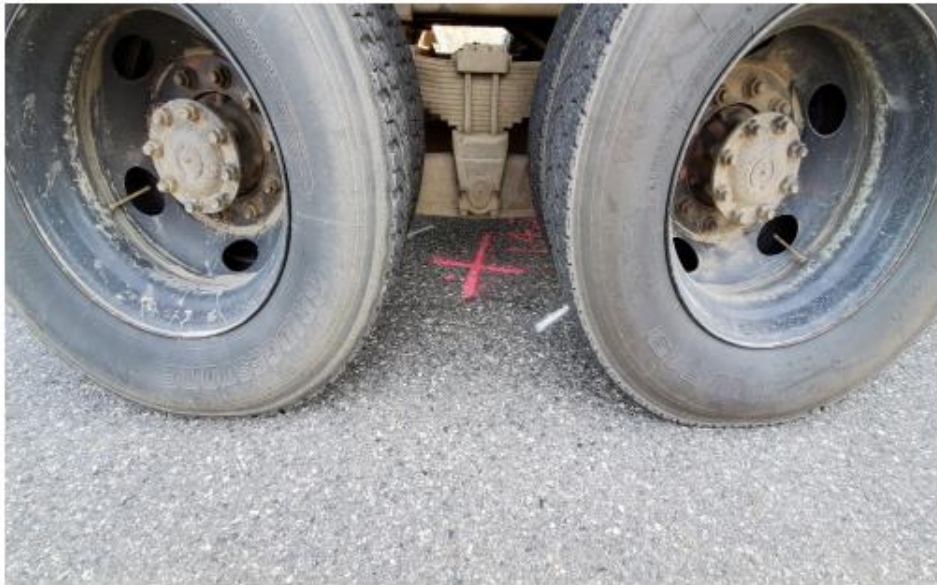
Picture 3. NBDTI Vehicle - Loaded Plow Truck at Static Location 9 – Rear Tandem Axles Centred over Crown.
