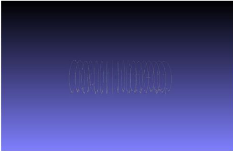
Figure 2. 18 LIDAR scanned cross-sections of a 5-metre section of CSP.
