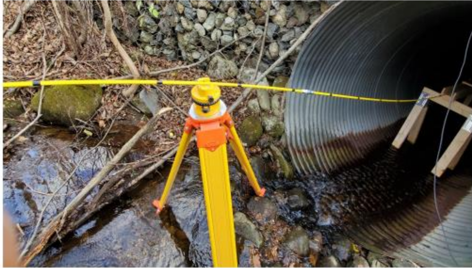
Picture 9. Tripod near the inlet of the CSP as a reference for incrementing the LIDAR between full scans.
