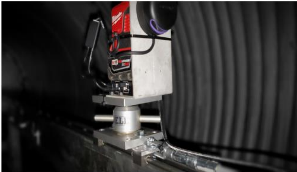
Picture 8. LIDAR mounted to railing system.
