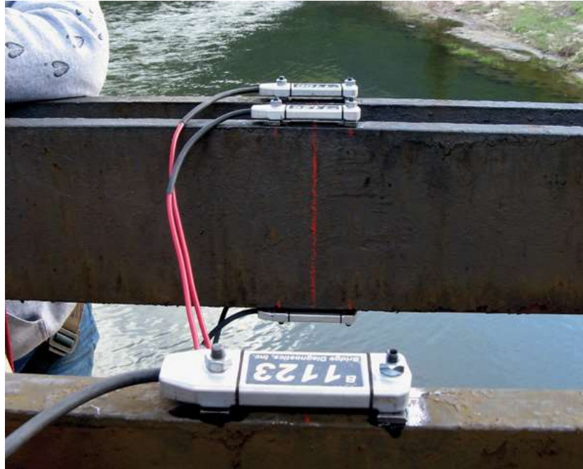
Figure 8 – Typical strain transducers installation 3
