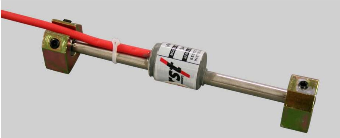
Figure 9 – Typical vibrating wire strain gauge 4
