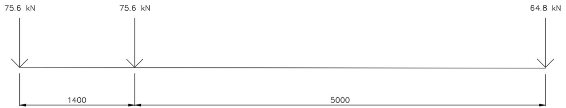
Figure 32 – Test truck axle configuration
