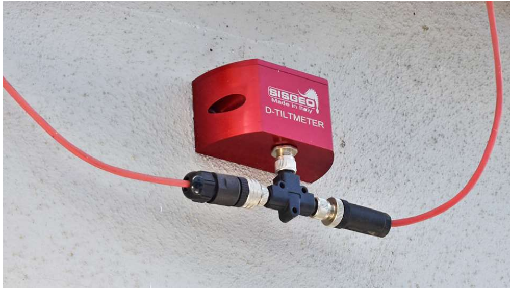
Figure 13 – Typical tiltmeter installation 8
