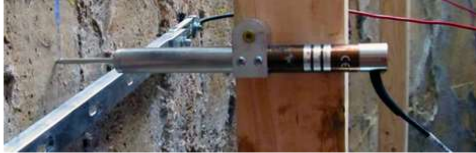
Figure 11 – Typical LVDT set up for displacement 6
