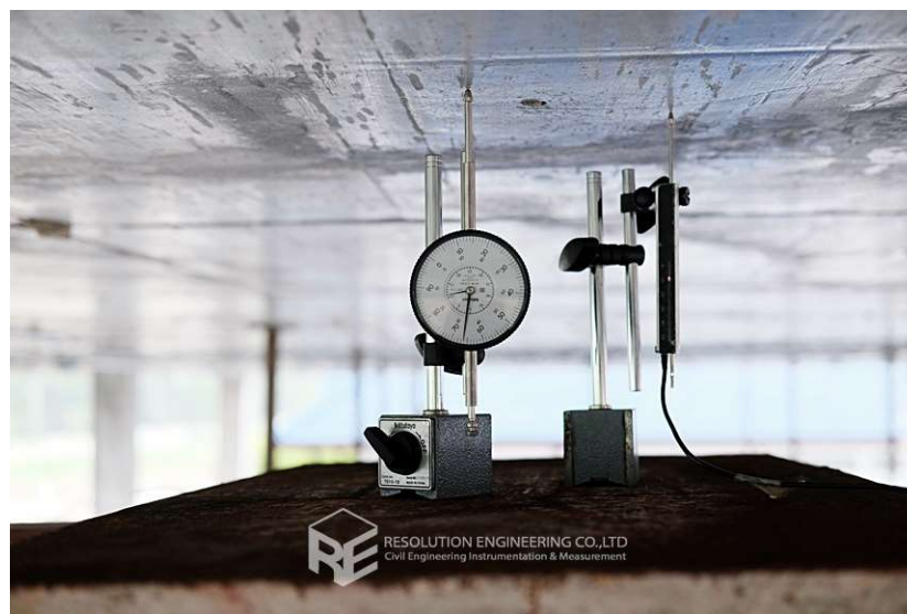
Figure 10 – Typical displacement dial gauge set up 5
