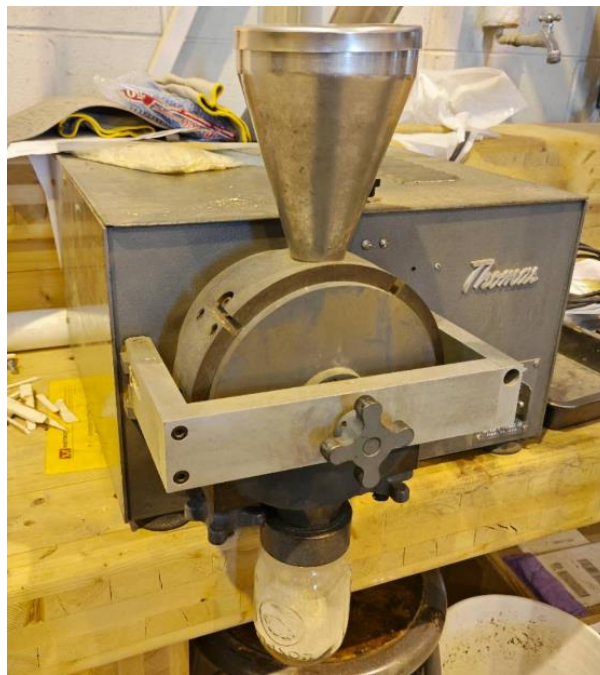
Figure 3.4 Wiley Mill grinder (Model: 3379-K05) used for pulverizing samples
