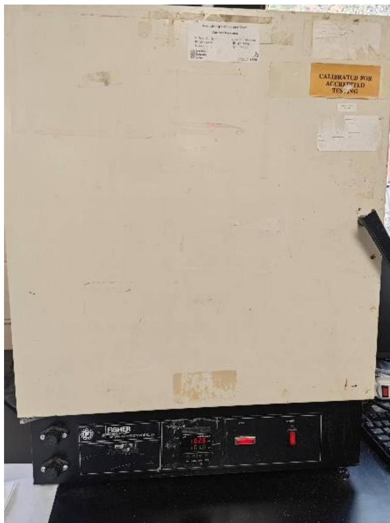
Figure 3.5 Oven (Model: 30F) with temperature control for drying samples
