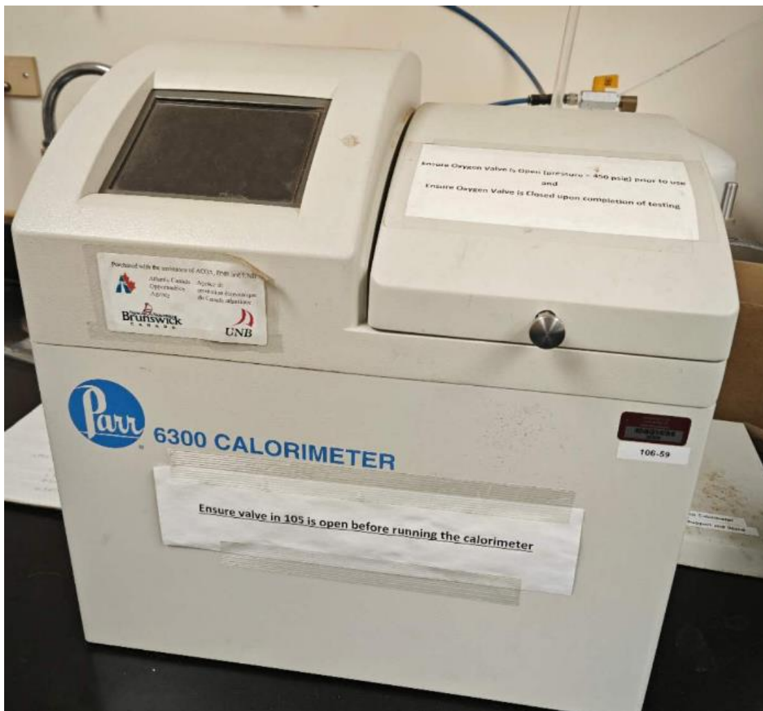
Figure 3.9 Automatic bomb calorimeter (Model: Parr 6300) used to measure the GCV of wood samples.
