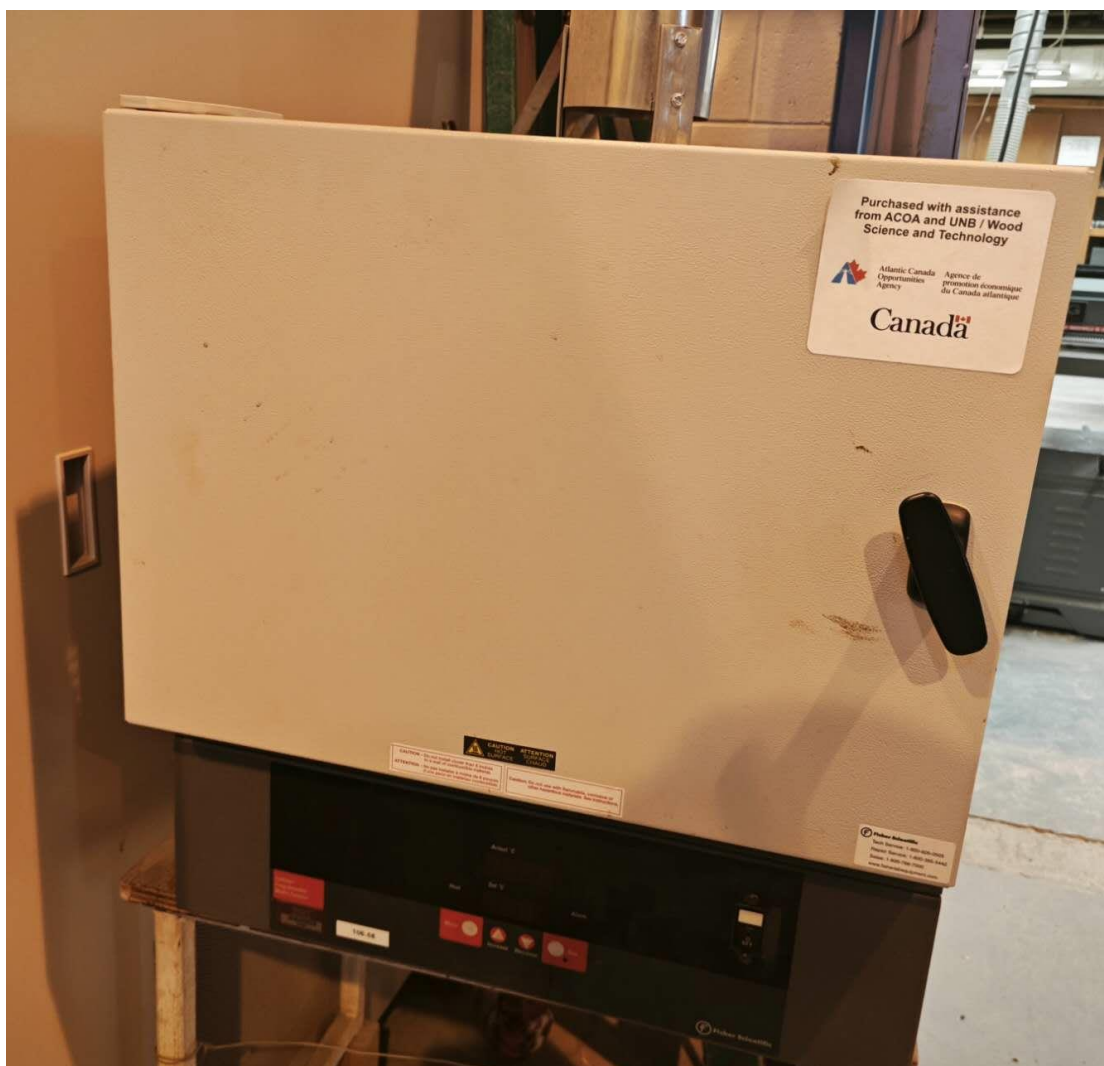
Figure 3.8 Muffle furnace (Model: Fisher Scientific 650-58) used for ash determination of wood samples
