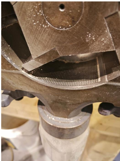
Figure 3.4 Wiley Mill grinder (Model: 3379-K05) used for pulverizing samples
