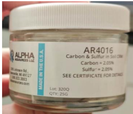
Figure 3.7 Certified reference materials used for calibration: AR4016 (C & S = 2.05%) and EDTA (AR2092)
