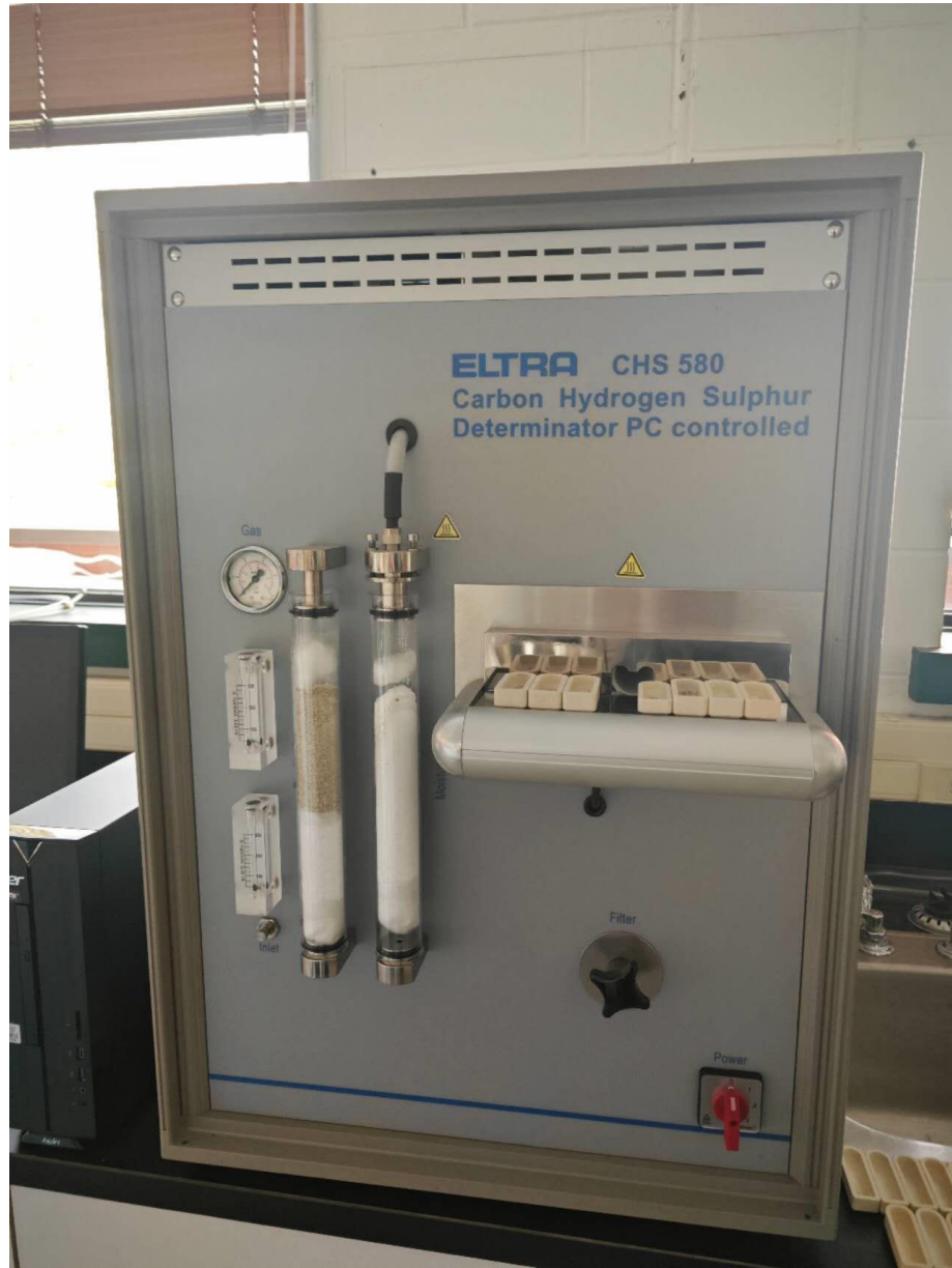
Figure 3.6 CHS analyzer (Model: ELTRA CHS 580) used for determining carbon, hydrogen, and sulfur content of wood samples
