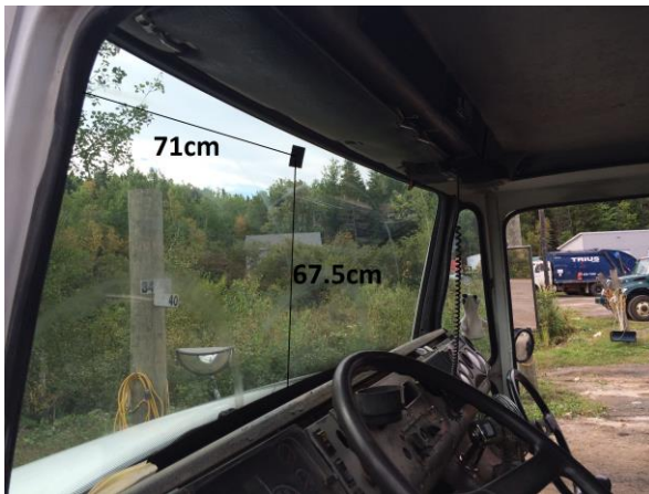
Figure 3.4. GoPro mounting position for windshield (standing/driving)
