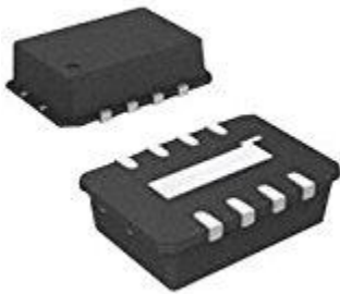
Figure 3.6. Tri-axial accelerometer (Analog Devices ADXL377Z)
