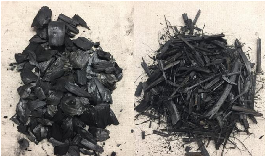
Figure 4.1: Softwood (left) and hemp (right) biochar samples
