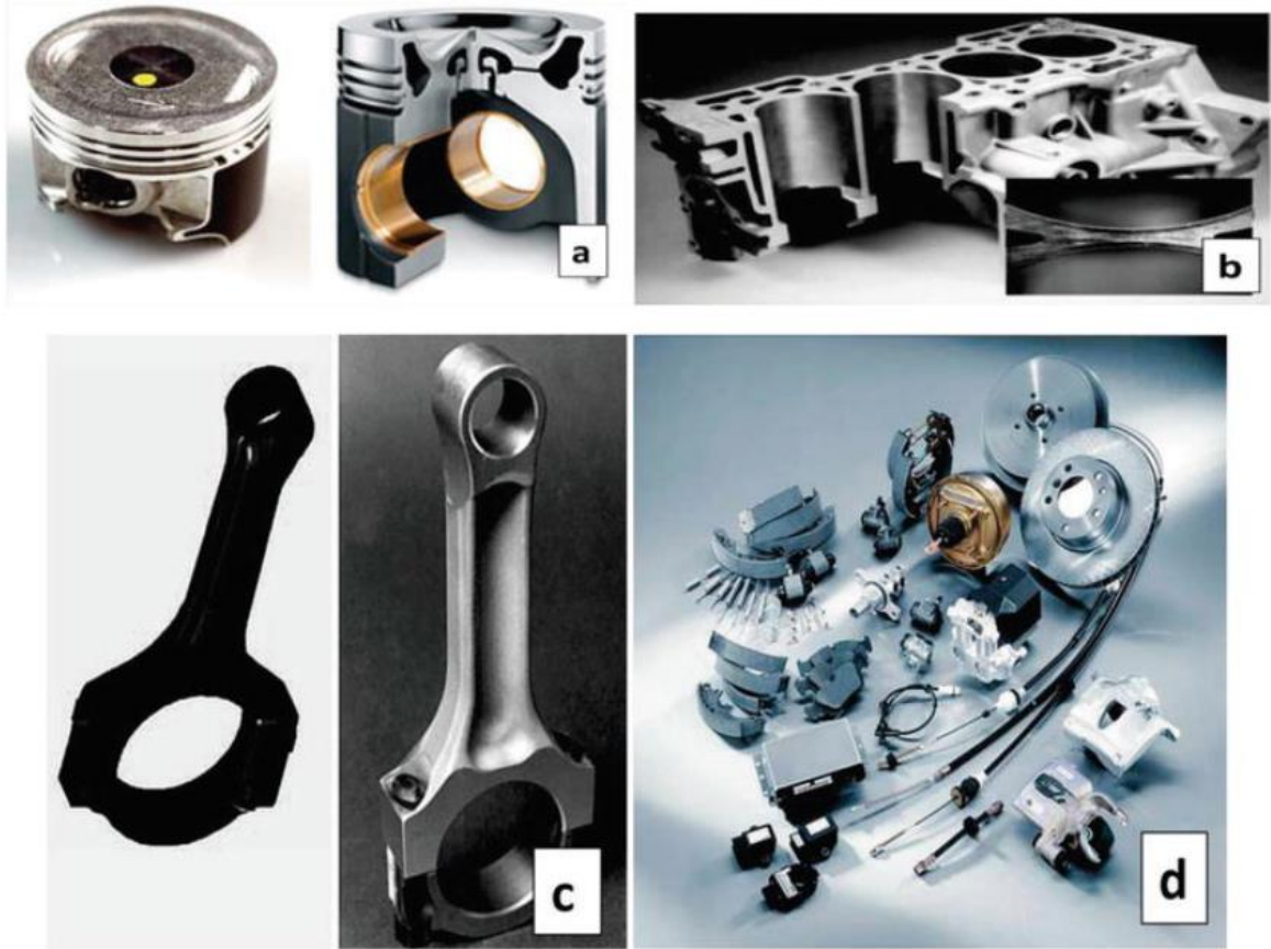
Figure 2.1: Aluminum metal matrix composite utilized in the making of (a) piston, (b) (b) cylinder barrel-equipped engine, (c) piston linking rod, (d) Braking mechanism [33].
