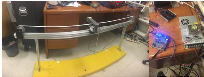
Figure 4.10: Fully View of Inverted Pendulum Test Setup with Control Circuit
