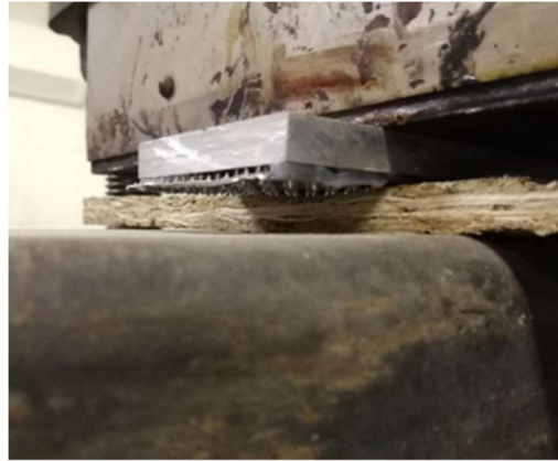
Figure 2.7 Pressing with the metal tooth-plate
