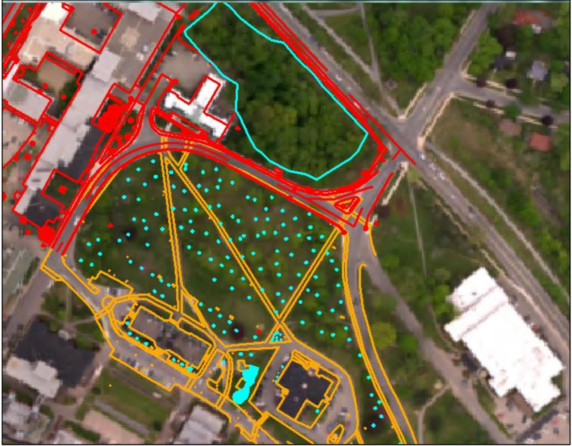
Figure 3.7: Example of the trees' points and the enclosed lines of the wooded area
