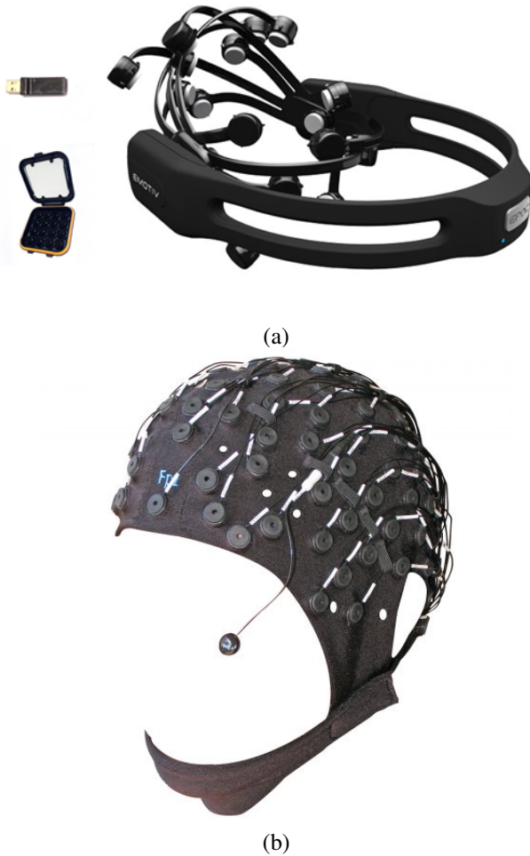
Fig. 4. EEG devices: (a) a 14-channel wireless Emotiv EPOC+ with accessories (b) 128 channel high-density EEG device.
