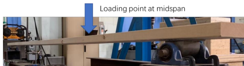
Figure 9 Experimental setup for measuring MOE of lumber
