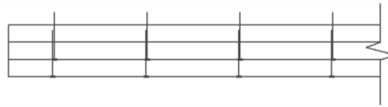
Figure 11 Nailing pattern of an NLT specimen (Front view)
