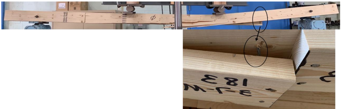
Figure 41 Segment slip accompanied with nail bended in specimen 3-7-M
