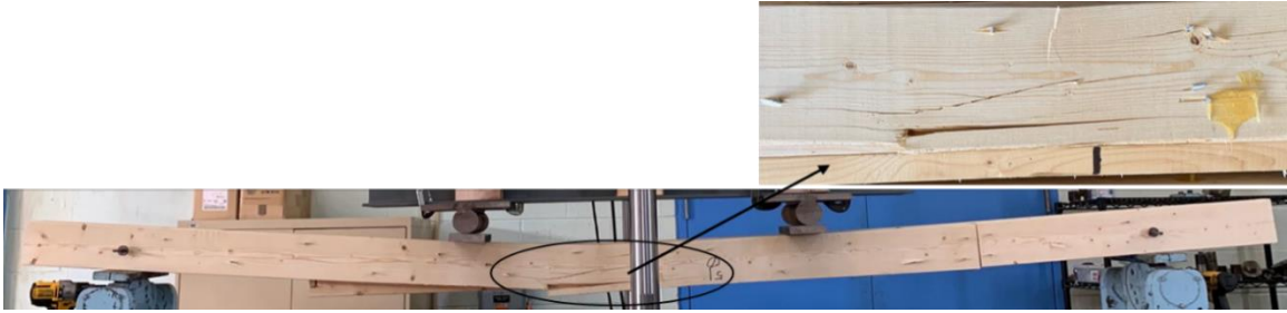
Figure 28 Simple tension failure occurring in specimen 3-7-H within the maximum bending moment area
