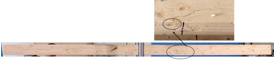
Figure 43 A knot existing at the location of failure in specimen 3-0-M
