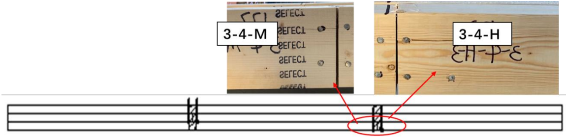
Figure 32 Splitting failure occurring in Type 4 specimens
