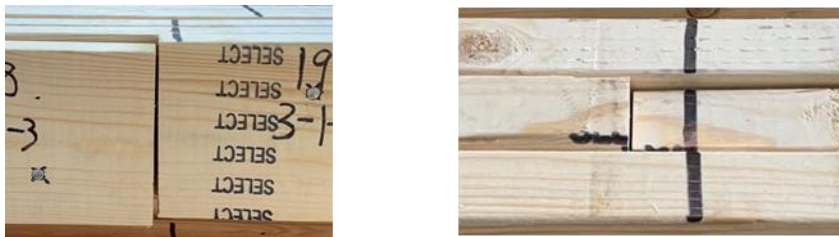
Figure 29 Slip between segments in Type 1 specimens
