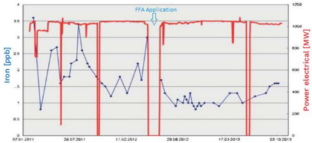
Figure 2.19: Iron reduction into steam generators in Almaraz Unit 1 [49]
