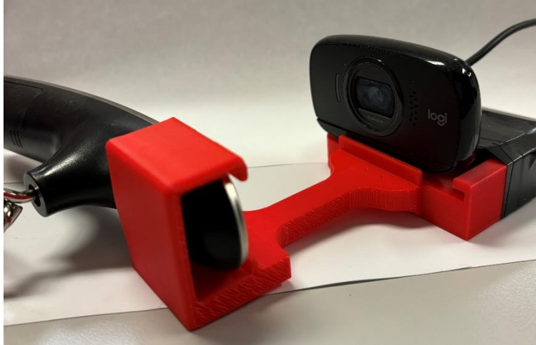
Figure 24: Camera mount for the luggage scale.
