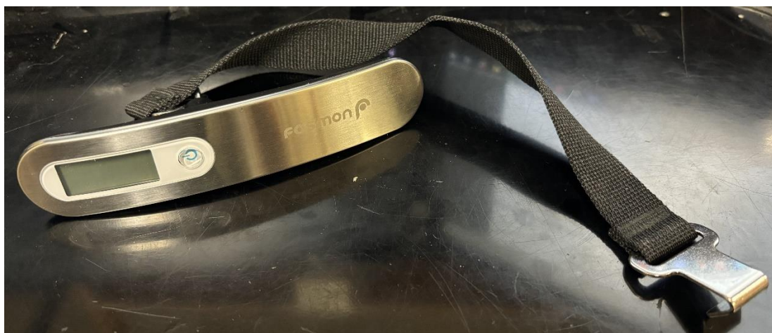
Figure 22: Luggage scale used for tension testing
