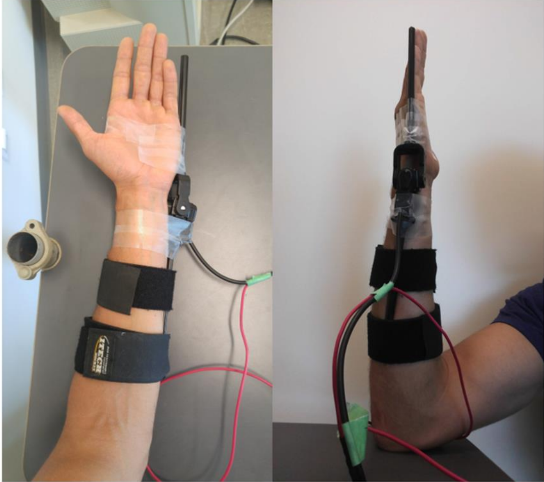
Figure 15 - Photos of electric goniometer placement on participant's wrists.
