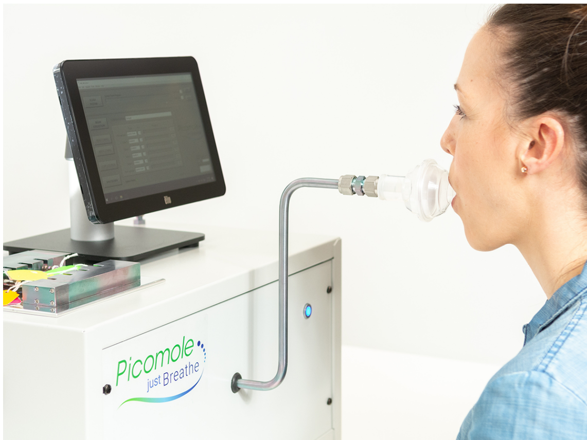
Figure 3.3: Usage of the exhaled breath sampler developed by Picomole Inc. [49].
