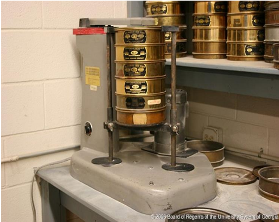
Figure 2. Typical set-up of stacked sieves on a mechanical shaker (Source: Prof. Susan Burns, Georgia Tech University, Department of Civil and Environmental Engineering)
