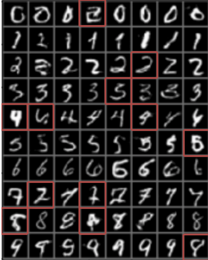
Figure 4.6: Untargeted white-box adversarial attack against adversarially trained MNIST classifier. Examples generated by the proposed attack. The defense was trained using PGD with \epsilon = 0.3 . The source classes are from 0 to 9. We performed the 500 step using Adam optimizer with learning 0.001, \lambda = 0.7 , and \epsilon = 0.05 . The red squares indicate failure in generating adversarial examples as decided by human labeling.
