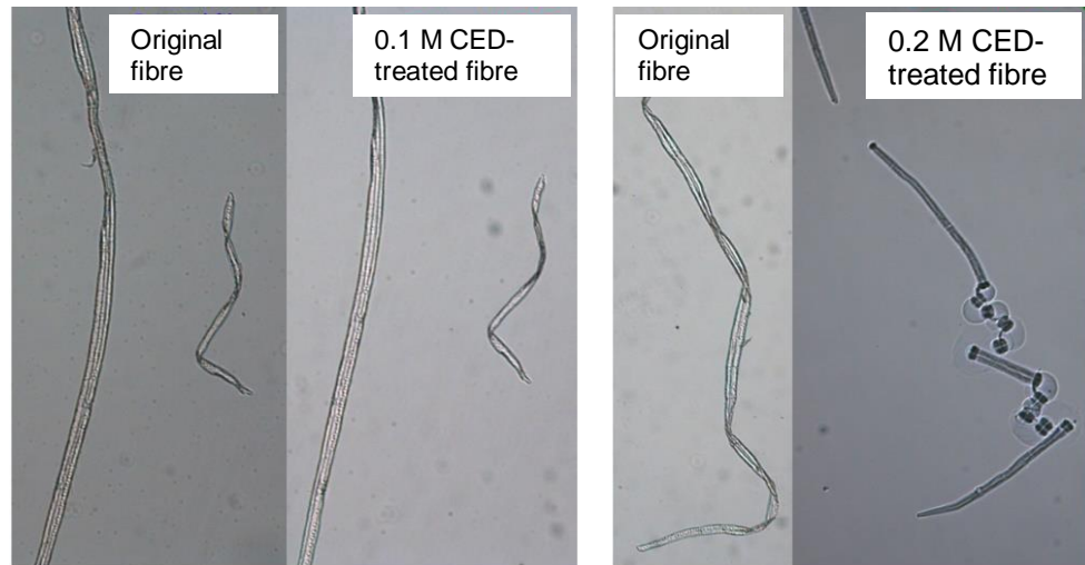
Figure 2.7. Optical microscopy images of original and CED-treated pulp fibres.
