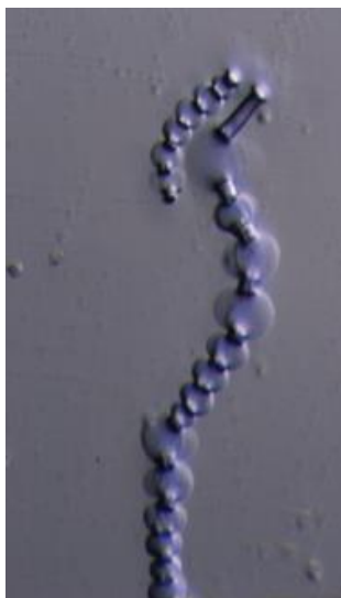
Figure 1.6. Intensive ballooning followed by total dissolution in 0.20 M CED solution.
