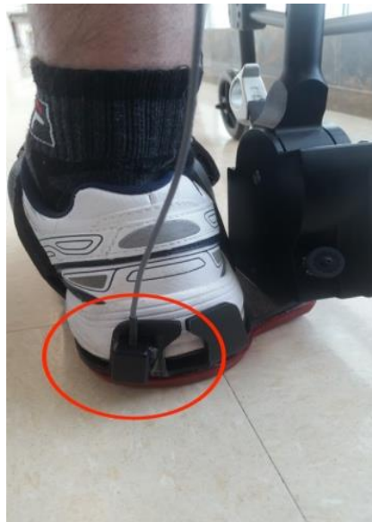
Figure 9. The accelerometer taped to the heel of the footplate to Ekso GT™.
