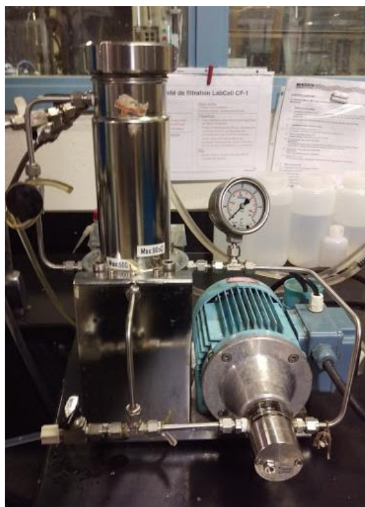
Figure 11: Membrane Filtration Column
