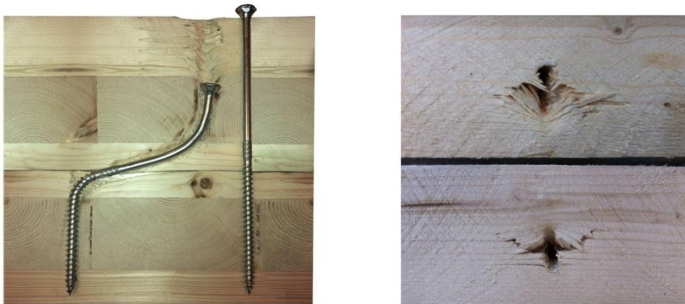
Figure 4-9: Observed failure for half-lapped connections without washers under shear loads (left) and tension loads (right).
