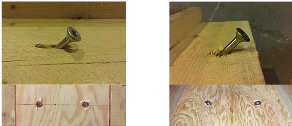
Figure 4-11: Observed failure for single-spline connections without washers under shear loads (left) and tension loads (right). Plywood has been removed to show the plastically deformed screws.
