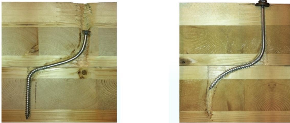
Figure 4-14: Residual deformations in half-lapped connections: without washer (left) and with washer (right).
