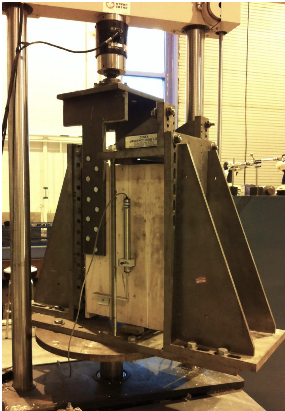
Figure 3-8: Photograph of shear test apparatus used for edge-to-edge connections.
