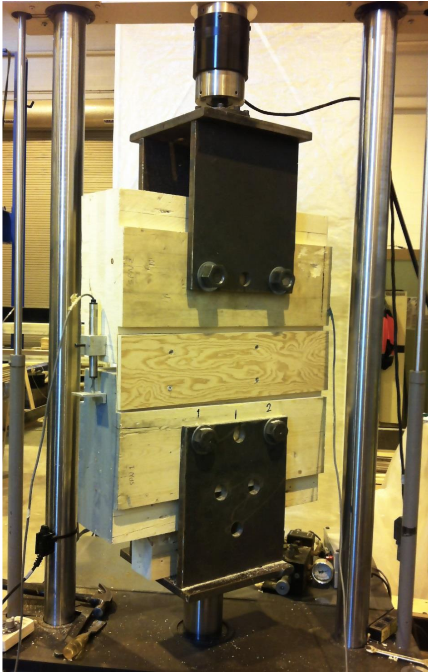
Figure 3-10: Photograph of tension test apparatus used for edge-to-edge connections.
