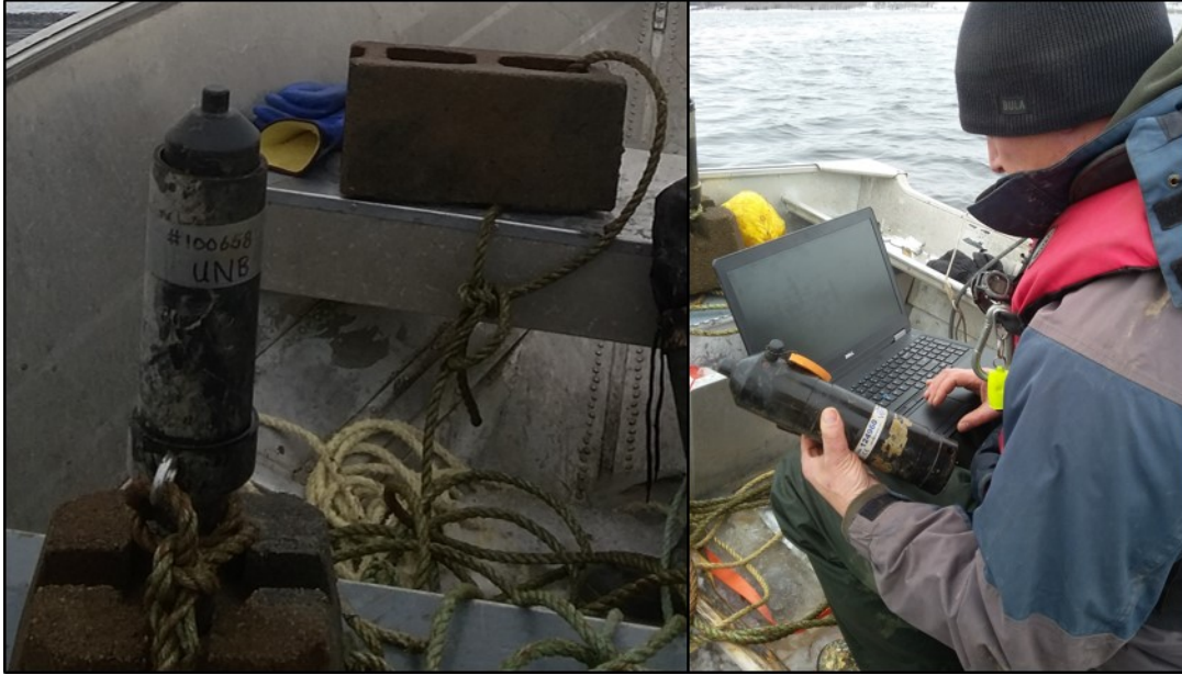
Figure 7: VR2W deployment setup (left) and data downloading (right).
