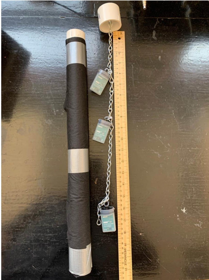
Figure 2-4: Example of PVC tubing used as hyporheic wells with temperature loggers suspended at 10 cm, 20 cm, and 40 cm from the cap.
