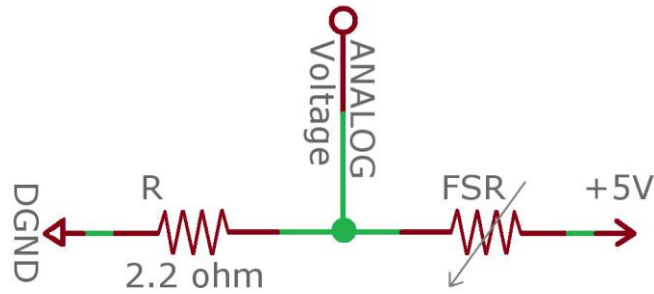
Figure 3. 6 – The circuitry used for reading FSRs data
