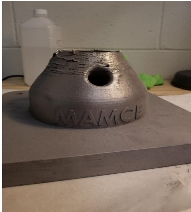
Fig. 4-2 Maraging steel failed test print piece
