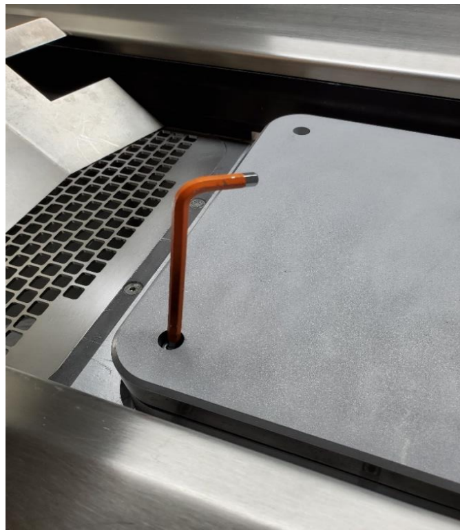
Fig. 3-3 Build plate bolt pattern
