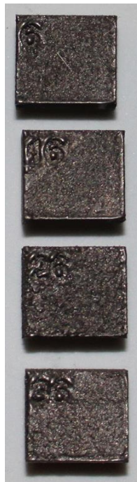
Fig. 4-6 Zoomed in samples 6, 16, 26 and 36. Surface roughness can be visually compared
