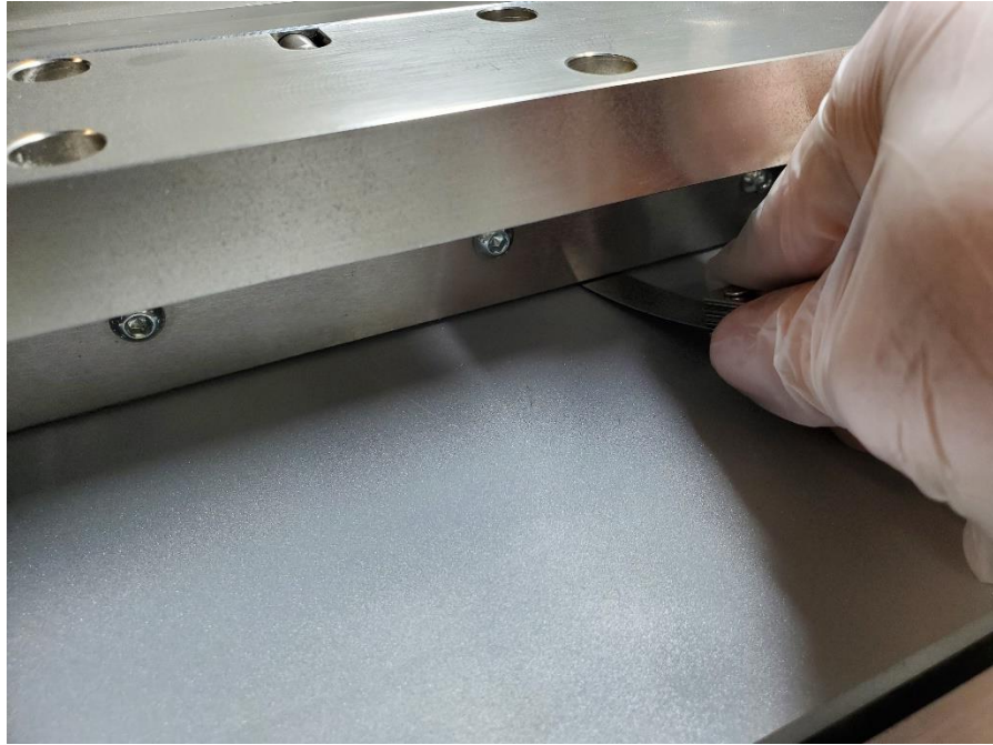
Fig. 3-4 Master recoater blade second zero check
