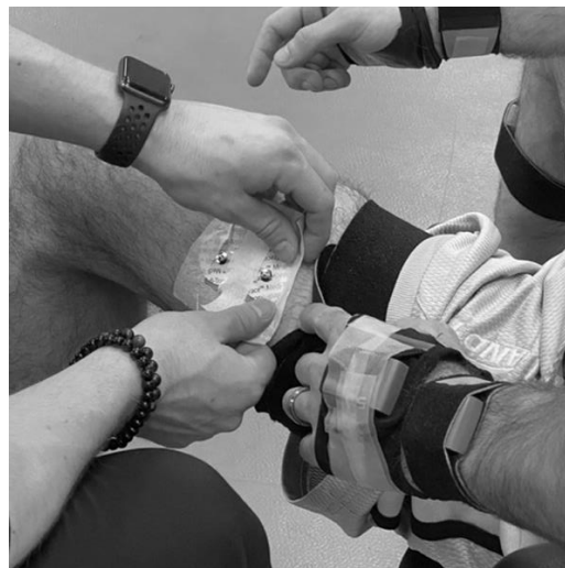
Figure 3. 2: EMG electrode placement for the vastus lateralis on an active Canadian soldier.
