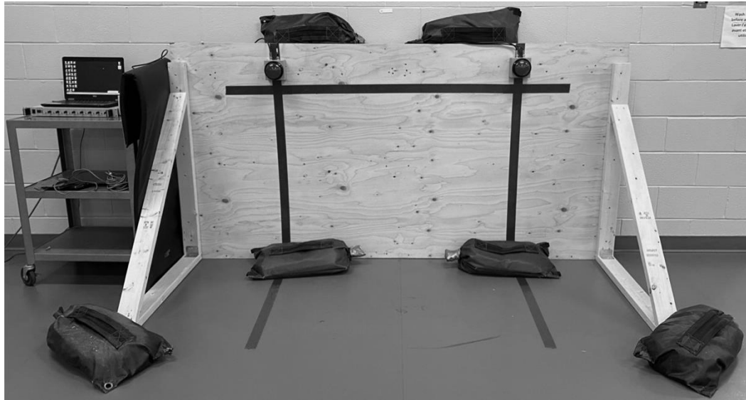
Figure 3. 1: Design and build of research equipment used to replicate the SBL test.
