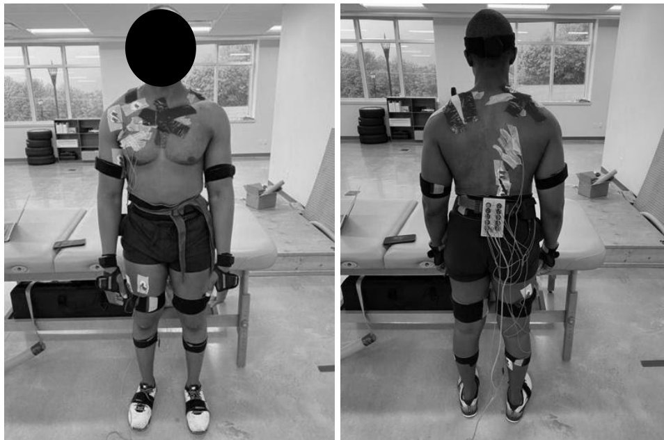
Figure 2. 2: EMG electrode and IMU participant setup
