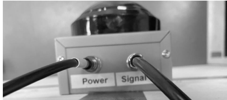
Figure 3. 9: Trigger to send 5V signal through EMG software to indicate placement of the lifting task.
