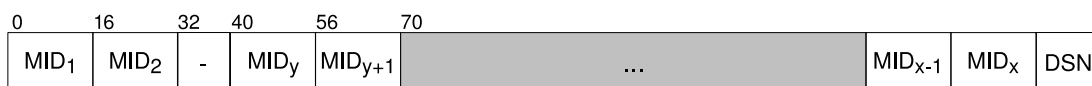
Figure 5.7: Bit structure of a D2 type DACK dissemination packet containing x acknowledgments consisting of a sorted sequence of MIDs and '-' characters. A MID_i - MID_k pattern indicates all MIDs between and including MID_i and MID_k are acknowledged.
