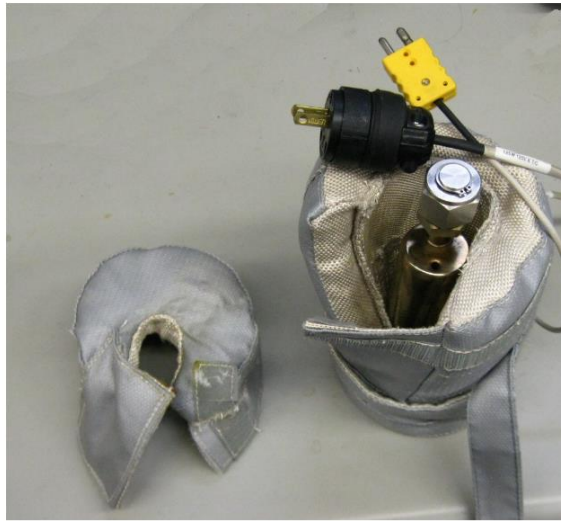
Figure 13. MOP canisters and the heating jackets inside which the canisters containing MOPs are heated, and the evaporated RE gases are fed into the ECR-PECVD chamber. The temperature is controlled using a K-type thermocouple [28].
