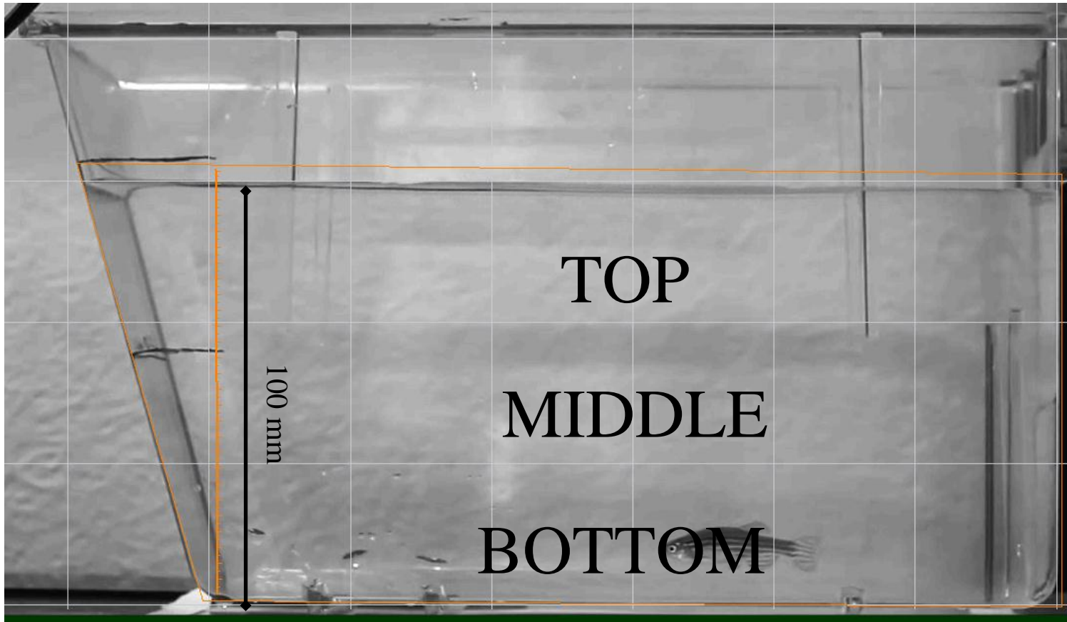
Figure 1: Apparatus used for the novel tank test. A 1.5 L tank (Aquabiotech Inc., Quebec) was virtually divided into a top, middle and bottom portion. The height of the water remained consistent throughout the experiments at 100 mm with a total volume 1300 mL of water.
