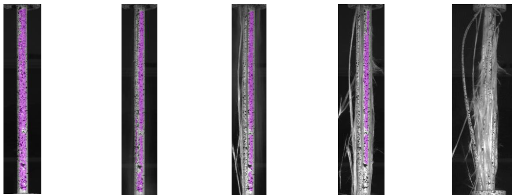
Figure 20- Failing mechanism captured by DIC
