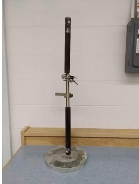
Figure 8- GFRP bar embedded in steel pipes curing
