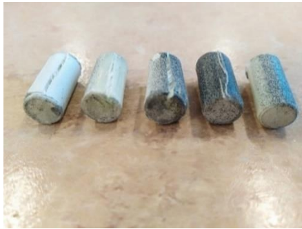
Figure 10- Failing mechanism in compression
