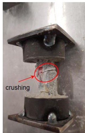
Figure 4- Failure mode in compression [6]
