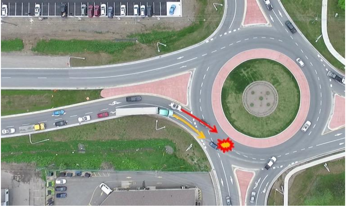
Figure 3.10: Failure to yield ROW to trucks
