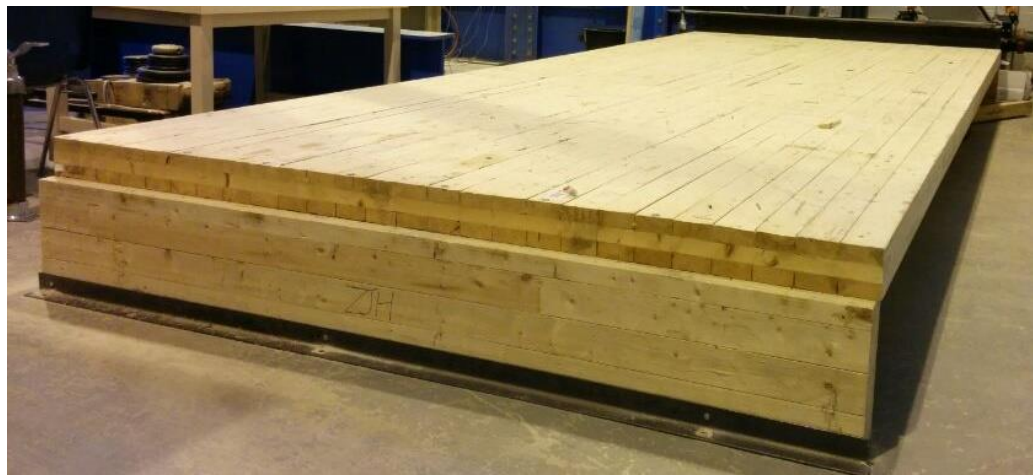
Figure 5.3 Support condition of a CLT panel
