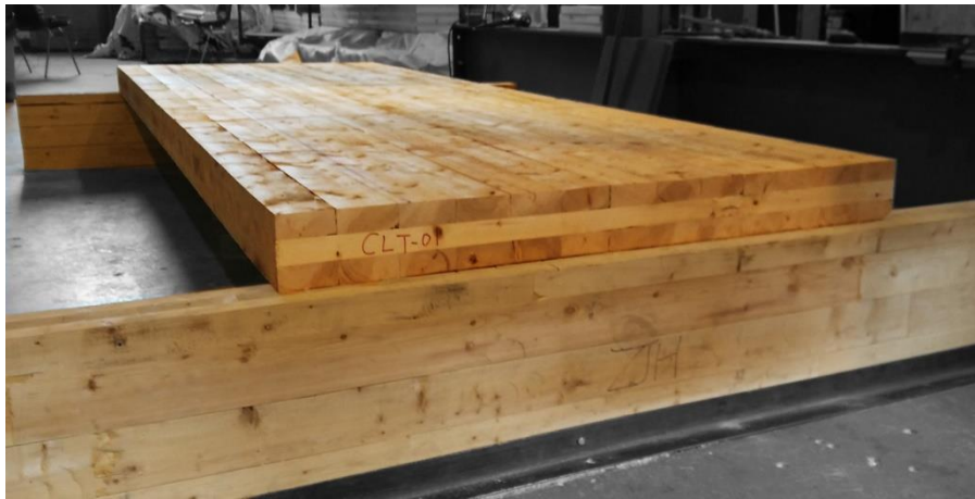
Figure 6.8 A CLT panel specimen under modal testing
