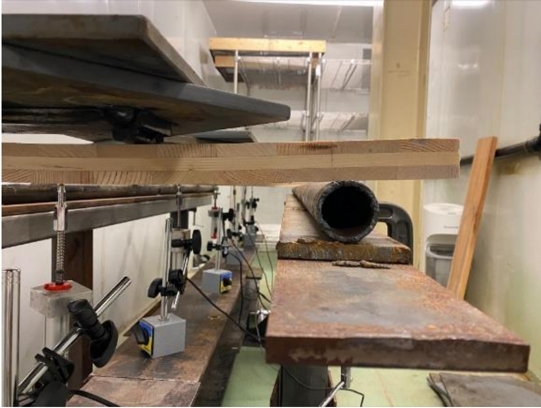
Figure 3.5 Supporting steel rod at the end of the loading span.
