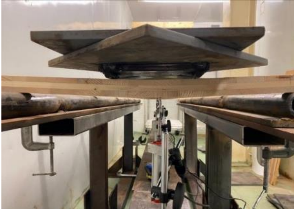
Figure 3.3 Creep test setup with an LVDT in the middle span of each specimen.
