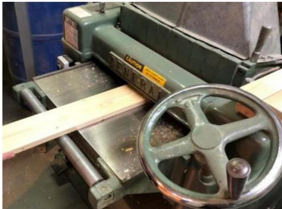
Figure 2.5 Ripping lumber using the heavy-duty bandsaw (upper) and planing wood strips to a given thickness using a planer (bottom).
