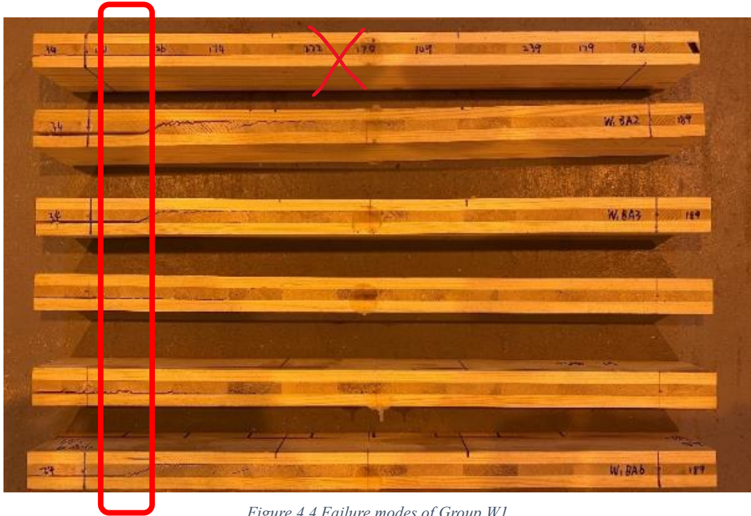
Figure 4.4 Failure modes of Group W1.
