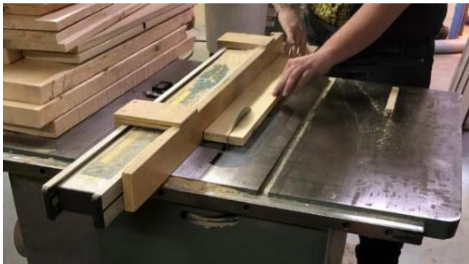
Figure 2.4 Cutting length using a circular saw (upper) and ripping width using a table saw (bottom).
