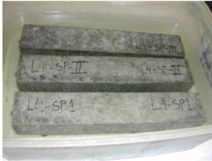
Figure 2.26: Sample in solution for MCPT (Latifee & Rangaraju, 2015)
