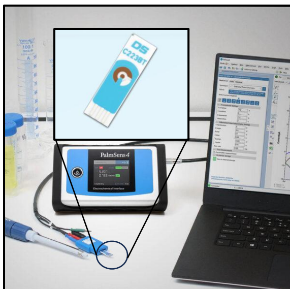
Figure 2.2. Experimental setup: a commercial gold SPE (Metrohm DropSens, C223BT) [95] connected to a potentiostat (PalmSens4).[96]
