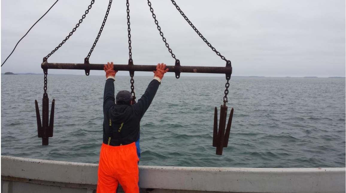
Figure 8: Custom made grappling hook used to retrieve lost lobster cages or other marine debris snarls.
