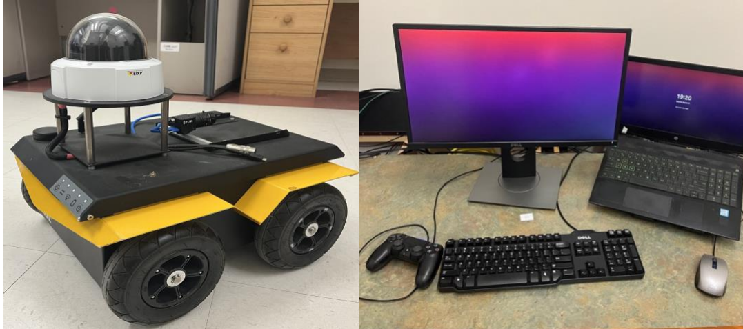
Figure 13: The jackal robot shown in the left picture. The system that the operator uses to control the robot is seen in the right picture.
